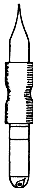
Fig. 46. Stopper for reaction tube with cap of drawn-out glass tubing. From Linderstrøm-Lang and Holter (1933b)
